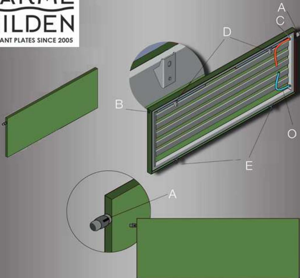
**步骤 4:** (a -b). 抬起暖气片并挂到支座支撑面上 (a -b).
